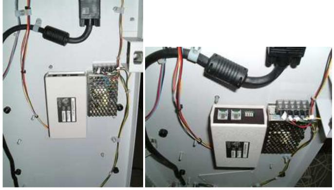
Please note the connections for the Telco Line In and To Fax are pointing up in the enclosure. There is a diagnostic LED next to the switch array that must easily be seen for diagnostics. This also makes the switches easy to get to for programming.
